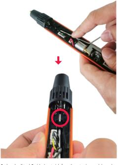
Push and pull tool. Residual materials from the extrusion module can be pushed out from the opening.
