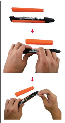
Use the unblocking tool to remove any residue within the white guide tube. Make sure that all the remaining residual filament has been removed from the guide tube, reinstall the back cover, and restart the feeding process.
