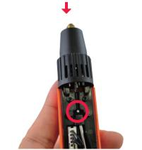
Press the tool slightly so that it is fully inserted into the feeding route. The tip of the tool will move about 1 cm through the round opening.
