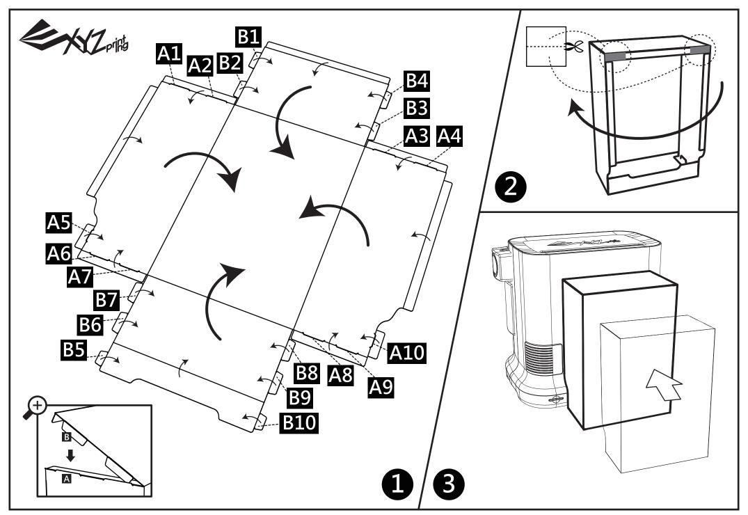
★ The components of extruder module will reach high temperature during operation, please always use the PET Protection cover before printing.
